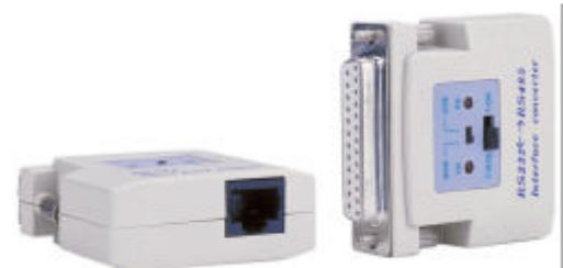
The *ic485-3* Interface Converter provides conversion between RS-232 interface and RS-485 standard. The RS-232 interface connection is via the unit's DB-25F female D-Type connector, while the RS-485 side's connection is via a five screw terminal block.
